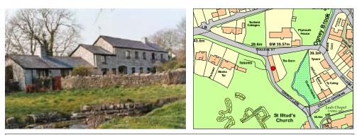
Outbuilding formerly of Plymouth House. Solid structure built of local stone, slate roof, stairs to the first floor, square headed openings with wide lintels. The building has been converted to a domestic dwelling. Mostly mid C19 - the building is shown on only part of this site on early 1840s Tithe Map. Stone walls and slate roofs.
