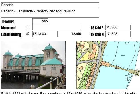
Built in 1894 with the pavilion completed in May 1929, when the landward end of the pier was rebuilt in concrete. Further rebuilding following ship collision in 1947. Approximately 200m long, and 15m wide at landing stage end. Central section on cast iron piles with wooden decking, landward and landing stage ends have concrete piles and decking.
