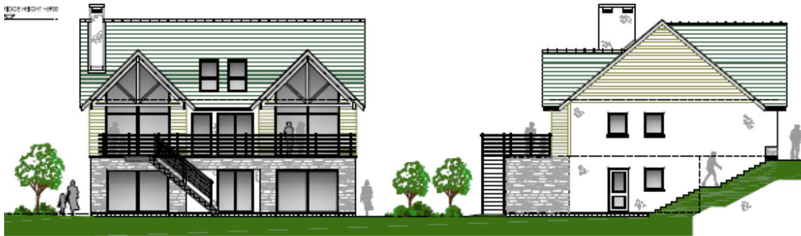
REAR ELEVATION HOUSE TYPE C
