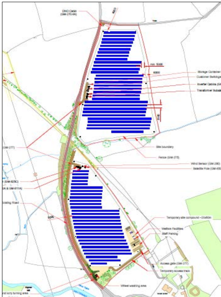
Figure 3 - Site Layout of Solar Farm
