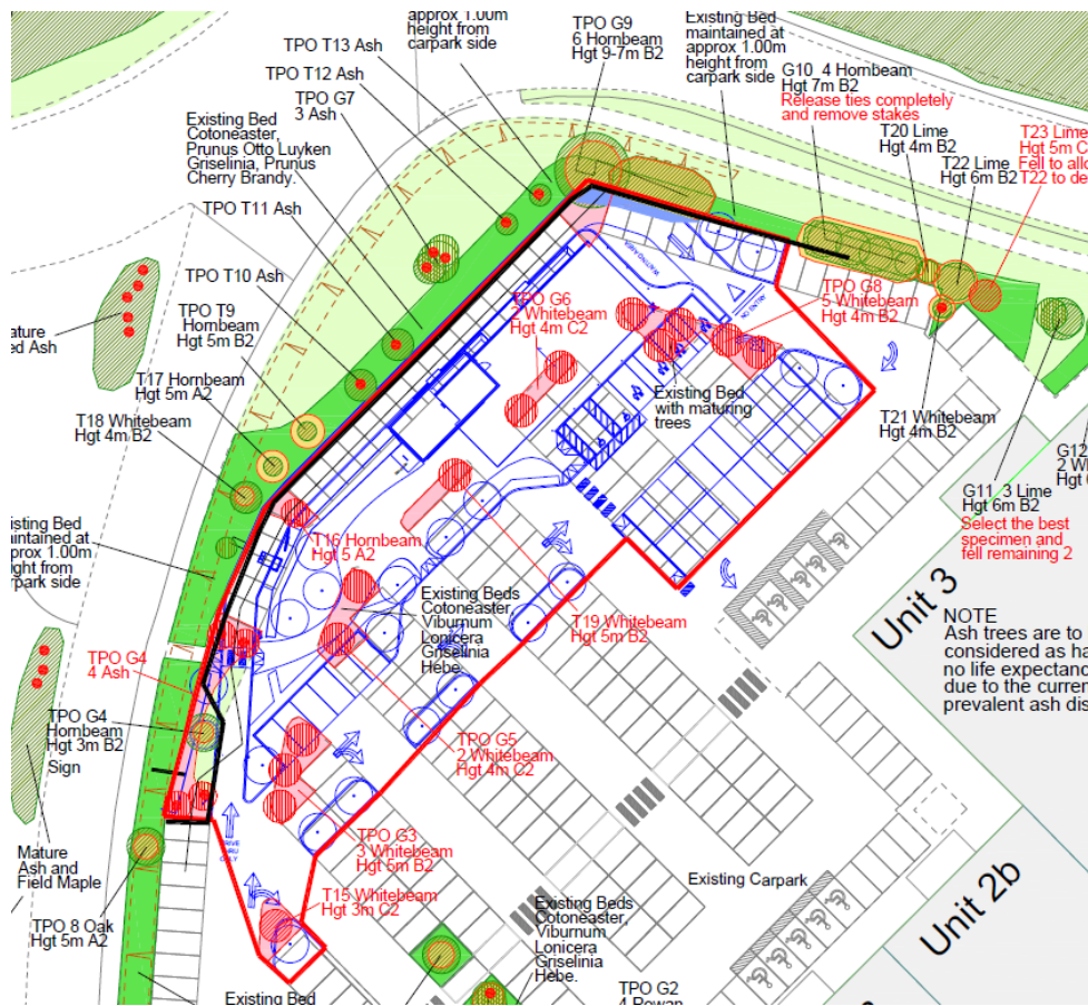
Plan indicating tree works to be undertaken with trees to be removed hatched in red and proposed tree planting indicating in blue
