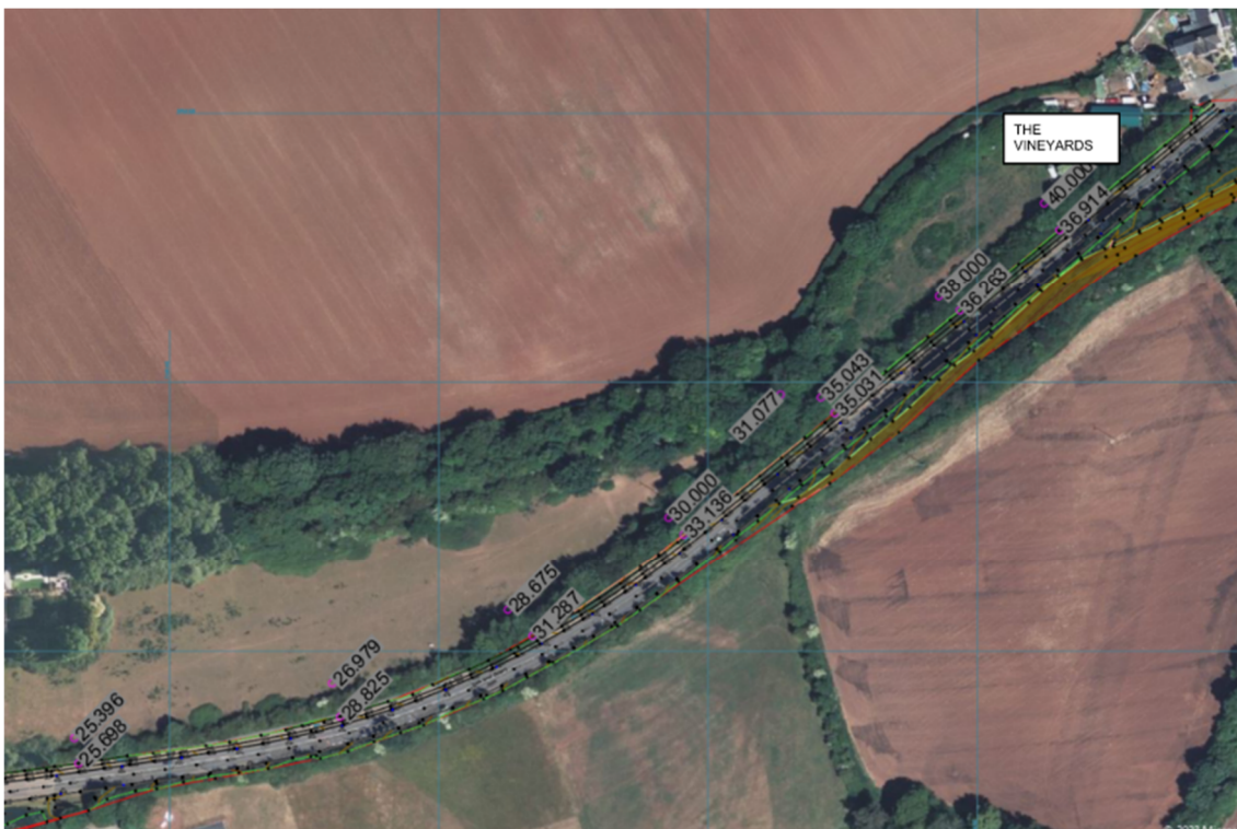
Figure 2: Existing Site elevation differences along Lavernock Road
