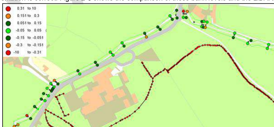
Figure 2-3: Comparison of 1D bank levels and LiDAR (difference shown in m)
