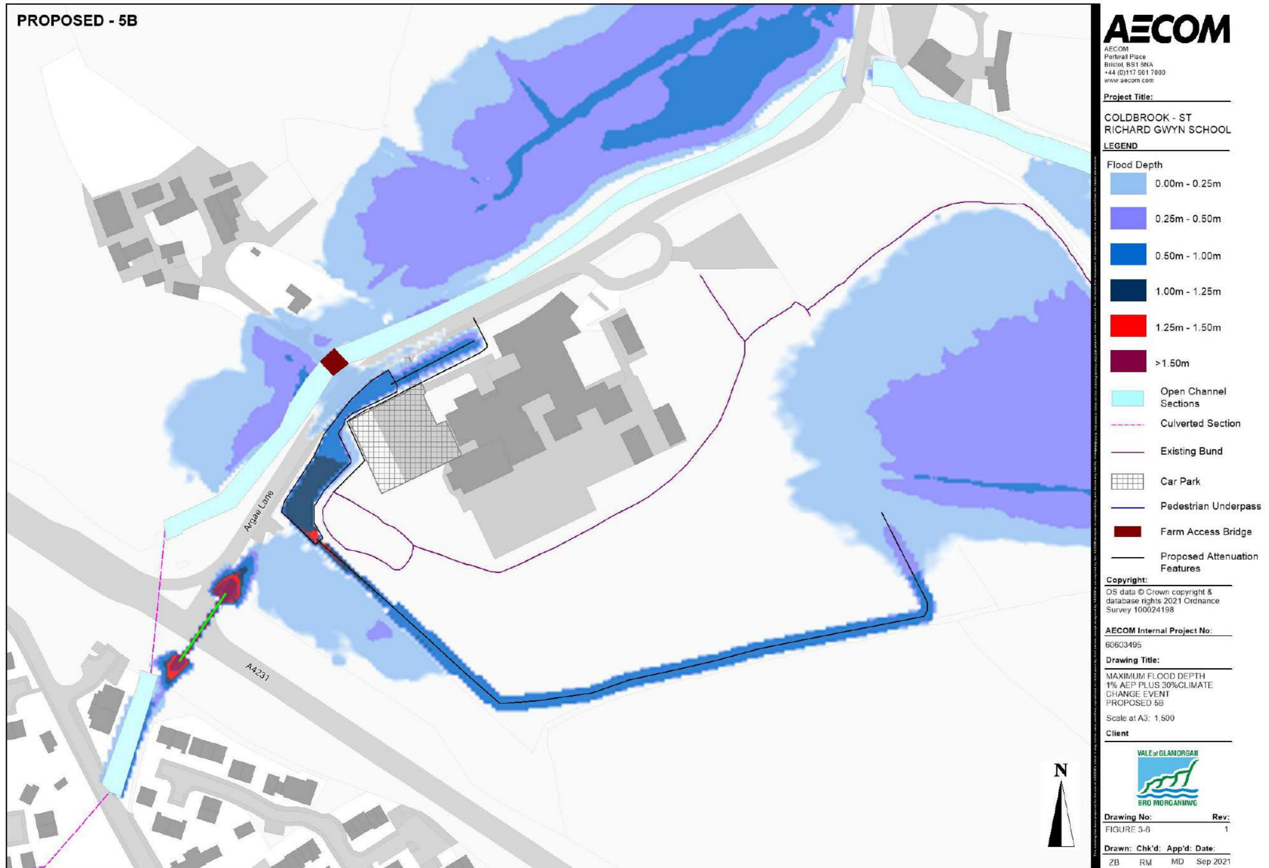
Figure 3-6: Maximum Flood Depth Map (Proposed) 1% AEP +30% Climate Change Event (Option 5b)
