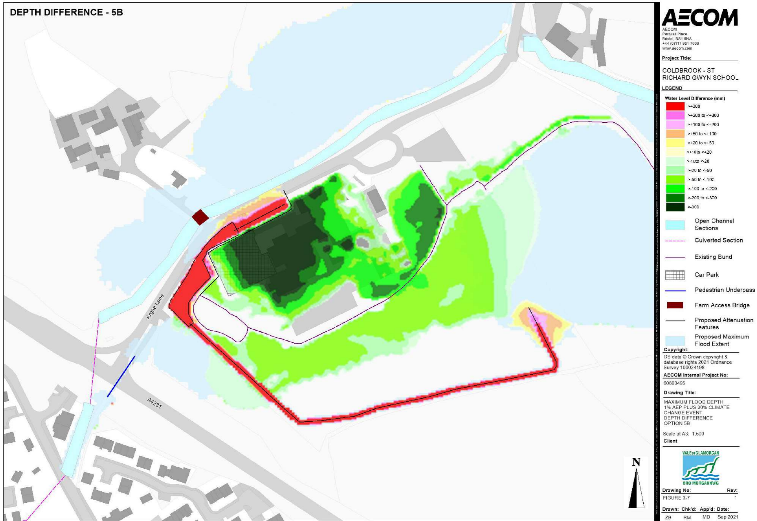
Figure 3-7: Depth Difference Flood Map 1% AEP plus 30% climate change (Option 5b)
