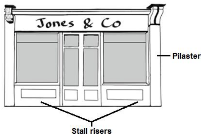
Figure 6: Example of a Traditional Stall Risers & Pilasters
