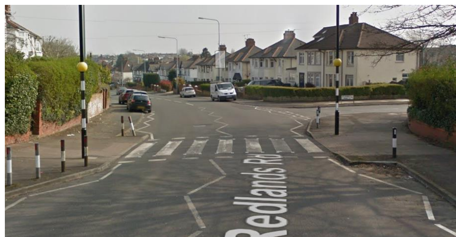
Dropped kerbs and tactile paving across junction with Hastings Avenue. Priority afforded to on-highway vehicles. Zebra crossing and narrowed carriageway for crossing of Redlands Road close to junction with Hastings Avenue and St Cyres Road.
